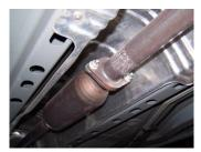
2. To remove stock exhaust, cut the muffler off near the overaxle tailpipe. Remove the rest of your stock exhaust, including resonator, at the 2bolt flange.
