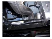
5. Slide the overaxle pipe onto the front pipe and insert the welded hanger into the rubber grommet.
